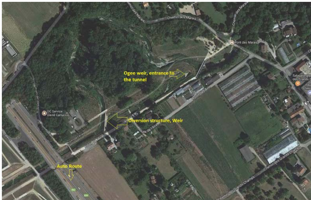
Figure 3 Newly constructed diversion structure and tunnel
